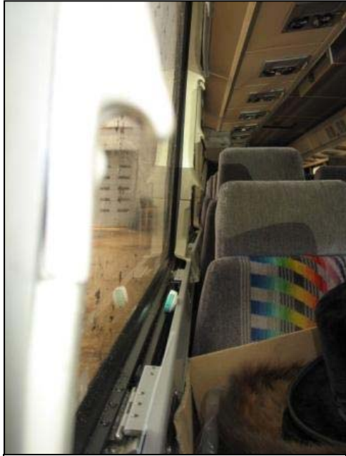
Figure 13: Rear view of the lateral intrusions along the right side of the interior.
