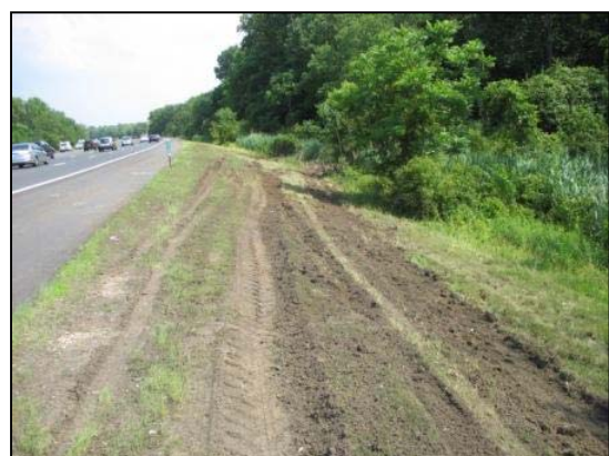
Figure 7: Trajectory and CCW yaw of the motorcoach across the roadside slope.
