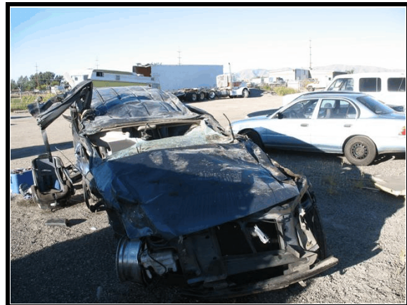
Figure 5. 2002 Mercury Mountaineer rollover damage
