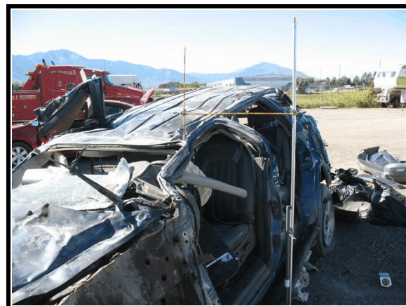
Figure 6. Maximum vertical crush
