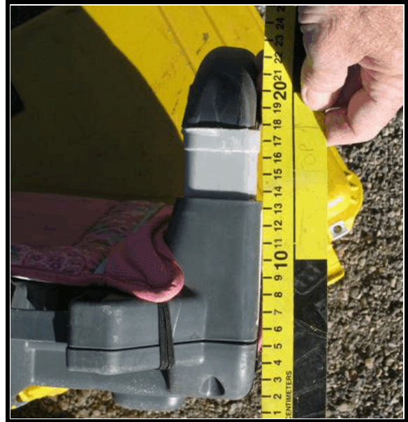
Figure 14. Stress marks to right arm rest
