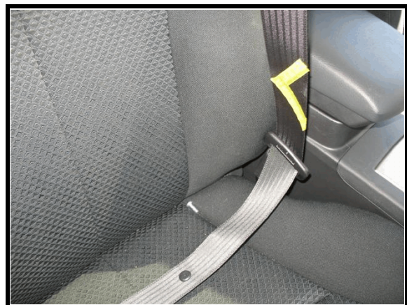
Figure 8. Front right occupant's safety belt showing load mark near the latch plate
