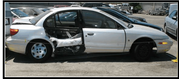
Figure 12. Right side damage, 2002 Saturn SL2
