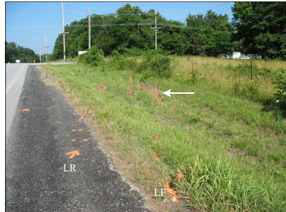
Figure 3: Roadway departure into ditch; arrow shows divot from front undercarriage impact
