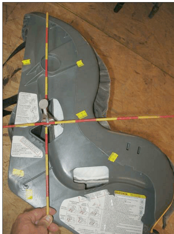
Figure 11: Yellow tape shows locations of small stress marks in the plastic shell
