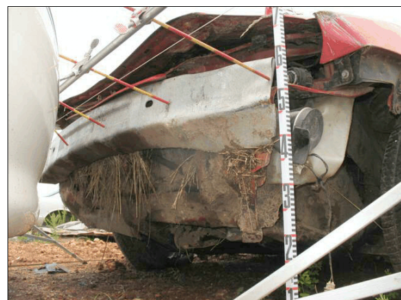
Figure 4: Damage on the Dodge's front undercarriage and bumper from the ground impact, each increment on the rods in 5 cm (2 in)
