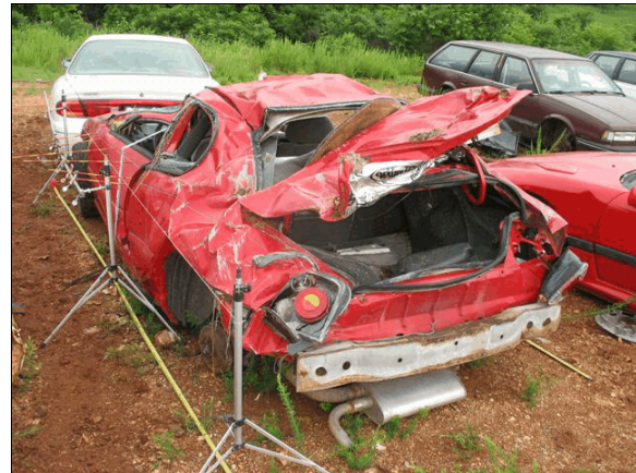
Figure 6: Damage on the left side plane and top plane from the rollover
