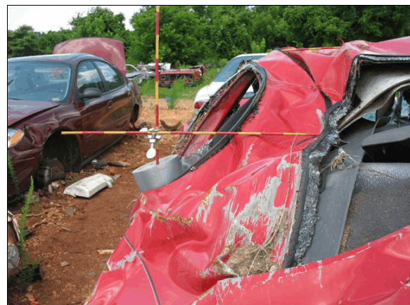
Figure 8: The maximum vertical and lateral crush from the rollover
