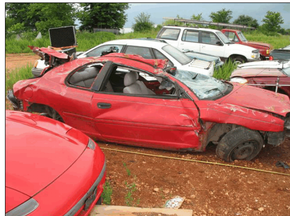
Figure 7: Damage on the top and right side planes from the rollover
