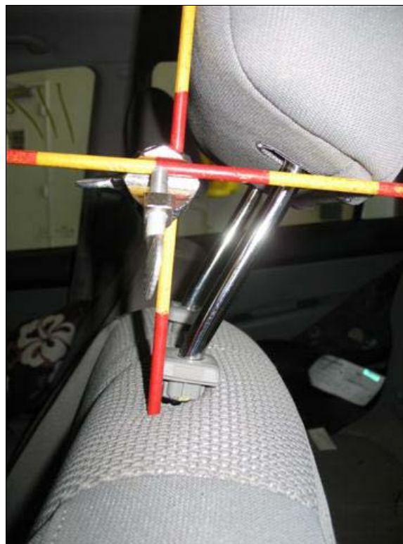
Figure 8: Driver's deformed head restraint
