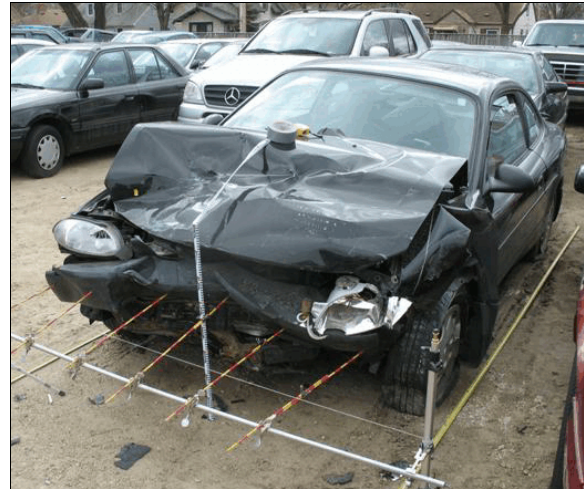
Figure 3: Damage on the front plane of the Ford from the impact with the back plane of the Kia
