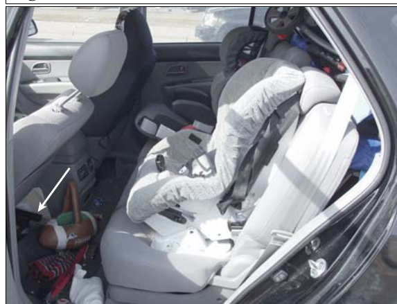
Figure 9: Police on-scene photo showing the position of the driver's seat back and the second row left CRS; driver's seat was moved to the full forward track position (arrow) when the child was removed from the vehicle; CRS in second row right seat position was not occupied at time of crash
