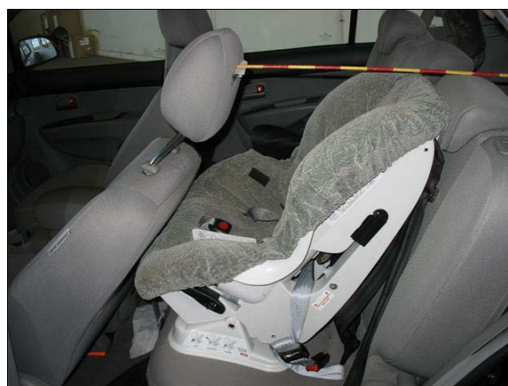
Figure 11: CRS placed in the Kia at the SCI inspection and driver's seat back positioned to contact the CRS; the distance from the head restraint to the back of the CRS was approximately 35 cm (13.8 in)
