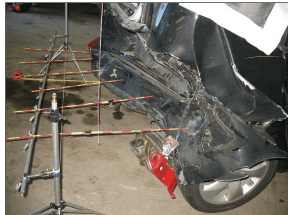
Figure 6: Right side view of the crush on the back bumper of the Kia
