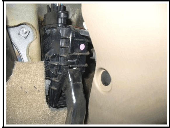
Figure 6. Denso accelerator pedal showing housing assembly
