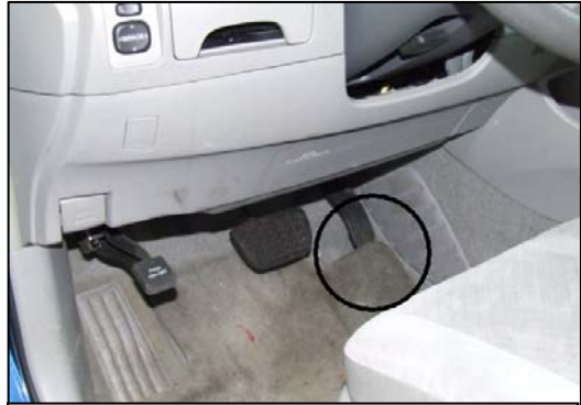
Figure 3: Post-crash position of the Toyota's OEM carpeted floor mat. Image supplied by the police investigator.
