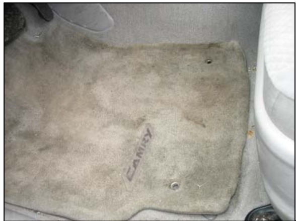
Figure 11: View of the unsecured OEM carpeted floor mat in the driver's foot well. Image taken during the SCI inspection.
