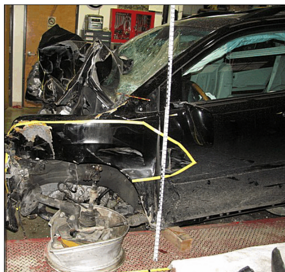
Figure 11: Damage on the left front wheel, suspension, and fender from the impacts with the guardrail posts
