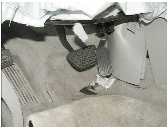
Figure 13: Condition of accelerator pedal, brake pedal, and floor mat at the time of the SCI inspection
