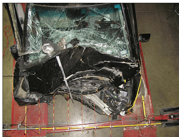
Figure 12: Top view of the front crush profile; the baseline is positioned 43 cm (16.9 in) short of the overall length due to the position of the vehicle on the hydraulic lift
