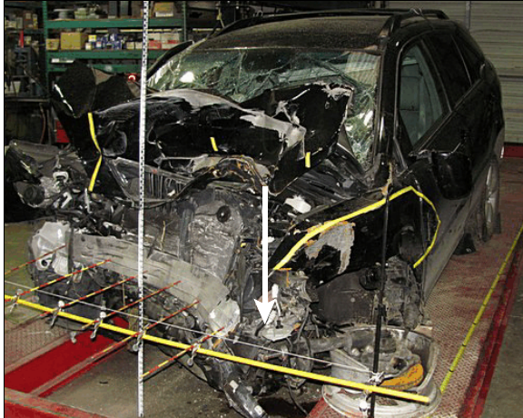
Figure 6: Arrow shows the area of impact with the guardrail posts on the front left corner; yellow tape shows extent of contact down left fender
