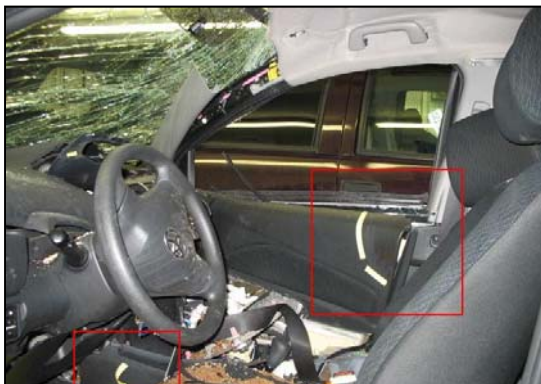
Figure 5: Left lateral view of Toyota's front row depicting the driver interior contacts.
