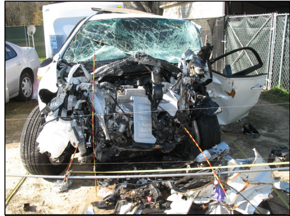
Figure 4: Frontal damage sustained by the Toyota.
