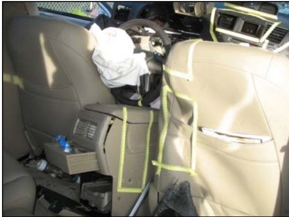
Figure 11: Right interior view of the passenger's contacts to the seat back and center console.
