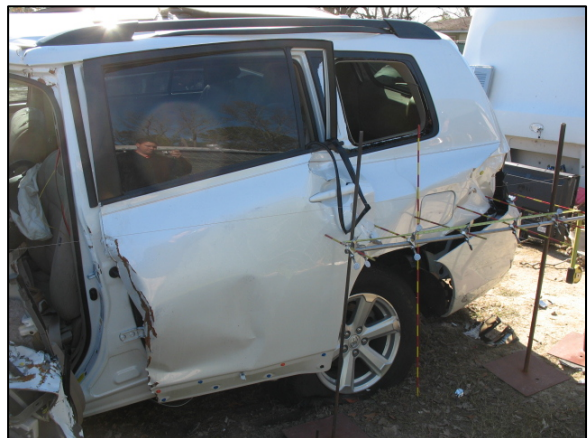
Figure 5: Left rear damage sustained in Event 3 impact.
