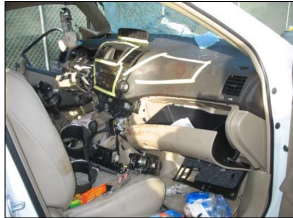
Figure 12: Right interior view depicting the passenger contacts to the center instrument panel.
