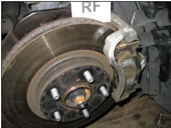
Figure 16: View of the condition of the Toyota's right front rotor.
