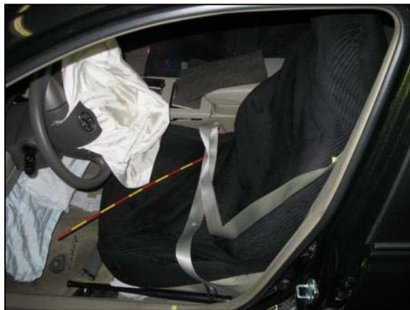
Figure 15. Deployed air bags in the Toyota Camry and the locked safety belt webbing due to pretensioner activation.
