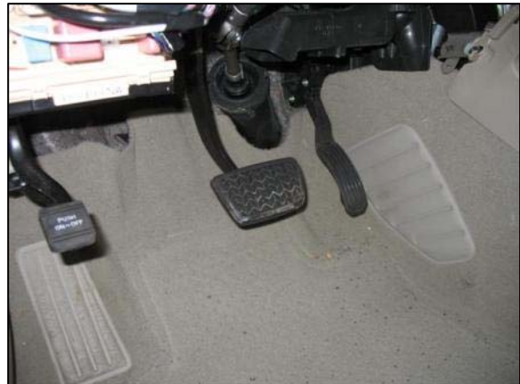
Figure 9. Floor, toe pan and foot controls of the Toyota Camry.
