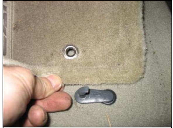
Figure 13. Positioning hooks of the OEM carpeted floor mats in the Toyota Camry.
