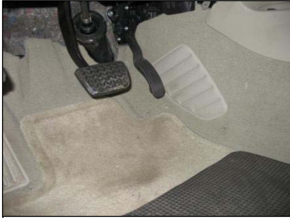
Figure 12. Overall view of the OEM floor mat in relation to the foot pedals in the Toyota Camry.
