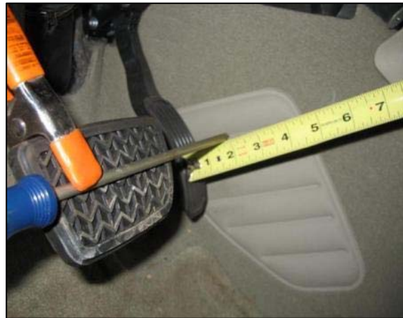
Figure 11. Height differential between the foot controls of the Toyota Camry.
