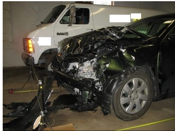
Figure 6: Oblique view of the Toyota's extent of crush.
