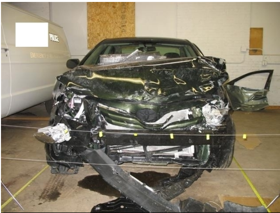
Figure 5: View of the Toyota's frontal damage.
