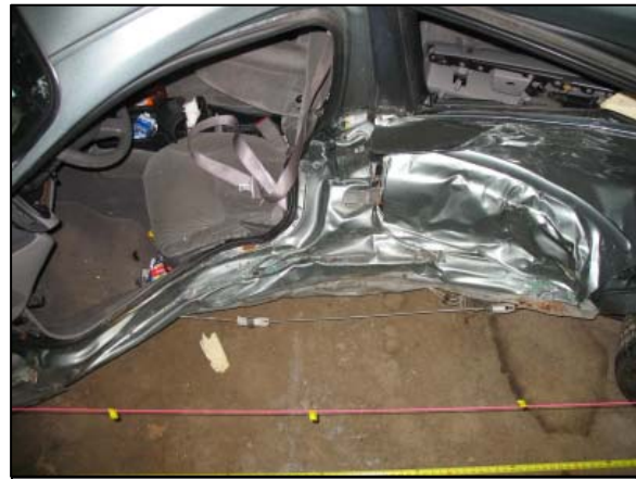
Figure 8: Overhead view depicting the Ford's extent of crush at the B-pillar.
