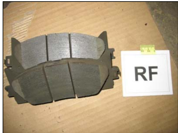
Figure 17: View of the condition of the Toyota's right front brake pads.
