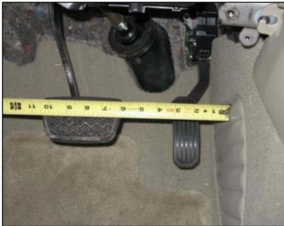
Figure 10. Lateral offset of the accelerator and brake pedals of the Toyota Camry.
