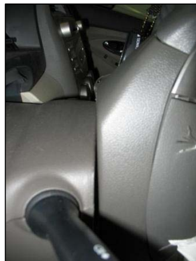
Figure 18. Deformed steering wheel flange of the Toyota from driver loading.
