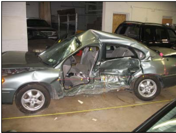
Figure 7: Left side impact damage of the Ford.
