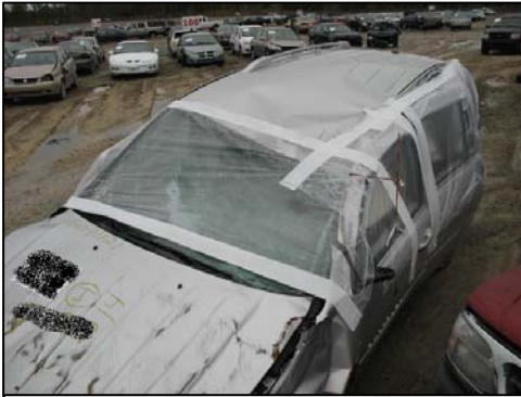
Figure 4: Overhead view of the rollover damage.
