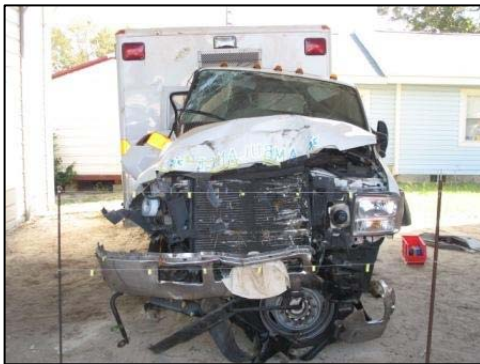
Figure 8. Tree impacts and resultant damage to the front of the ambulance.
