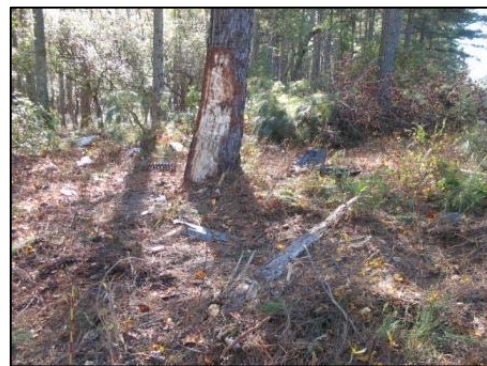
Figure 7. 46 cm (18 in) diameter tree struck by the right side of the ambulance.
