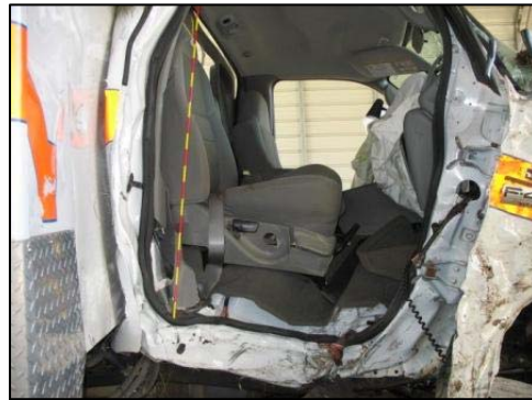
Figure 13. Exterior view of the intrusion into the front right passenger compartment.
