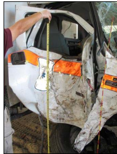
Figure 10. Damage to the right front door area.
