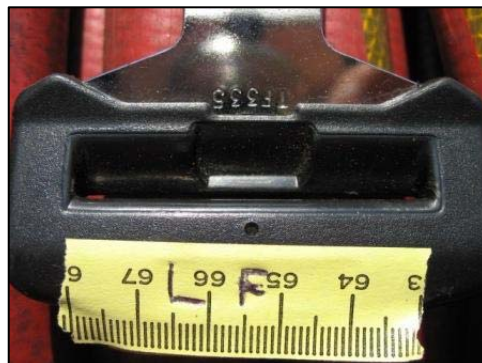
Figure 17. Frictional abrasion across the driver's latch plate.
