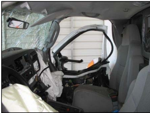
Figure 12. Intrusion of the front right passenger area.
