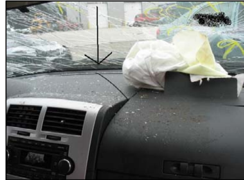
Figure 8: Left wire glove compartment door spring protruding from IP.
