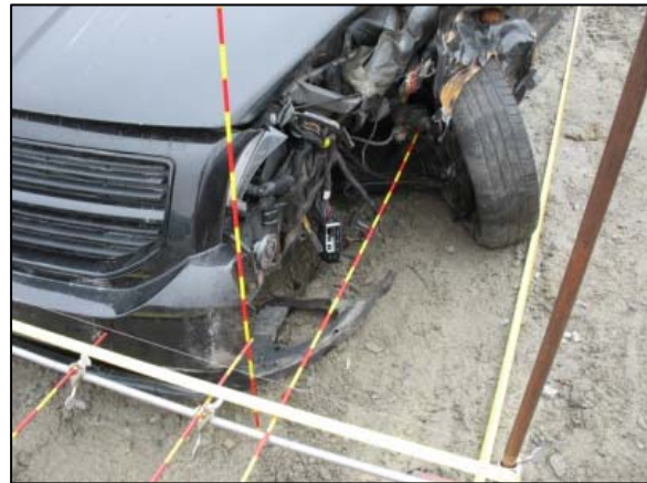
Figure 7: View of the direct damage along the Dodge's left side.
