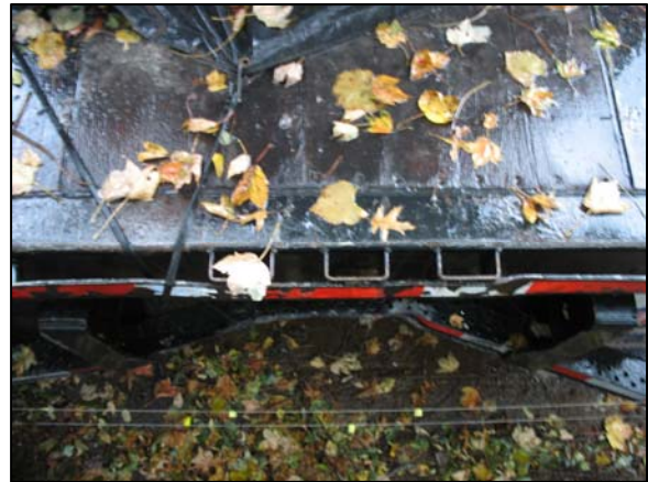
Figure 8: Overhead view of the deformation of the center aspect of the guard.
