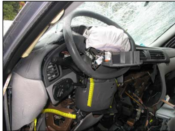
Figure 13: View of the steering assembly deformation.
