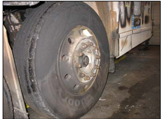
Figure 8. Fire damage to the left tag axle tire.
