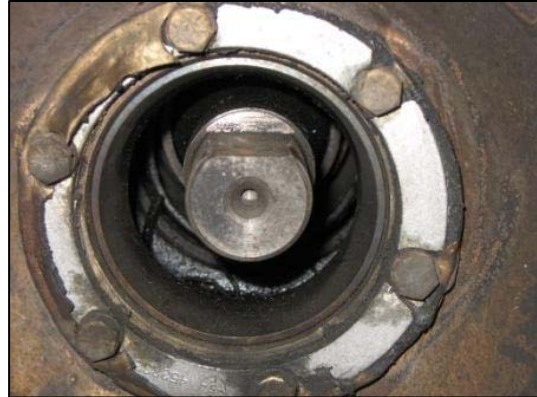
Figure 12. Close-up view of the wheel bearing races with the seals, tapered roller bearings and inner races missing.
