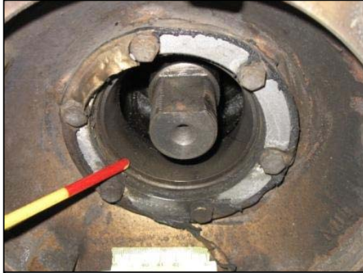
Figure 16. Damaged wheel bearing of the right tag axle.
