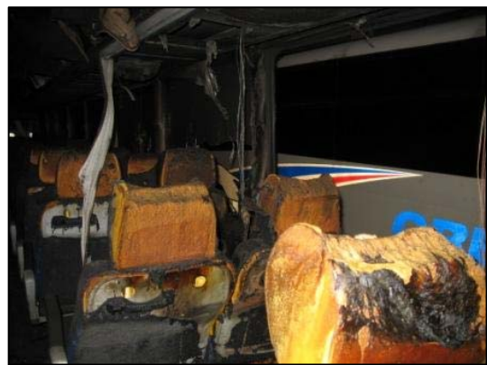
Figure 15. Fire/heat damage to the right row seatbacks.
