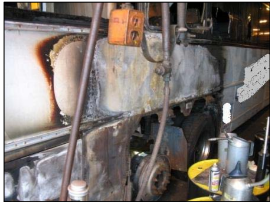
Figure 5. Right side fire damage over the rear axle areas.
