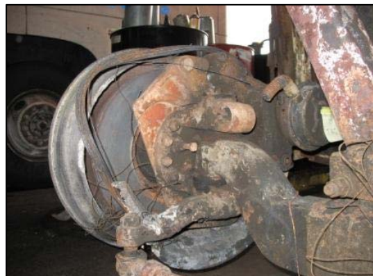
Figure 13. Undercarriage view of the right tag axle brake assembly and the melted alloy wheel.
