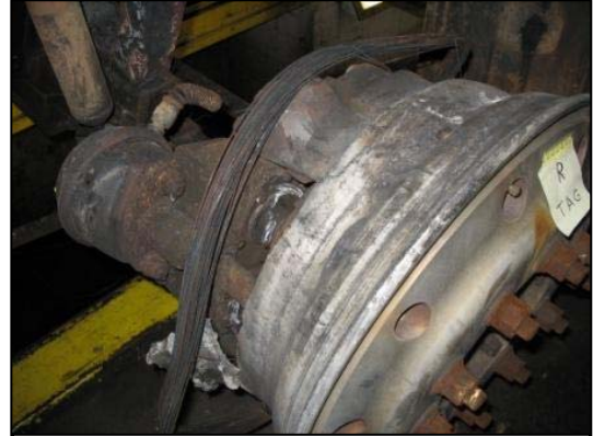
Figure 17. Fire damage to the right tag axle alloy wheel and the remnants of the tire.
