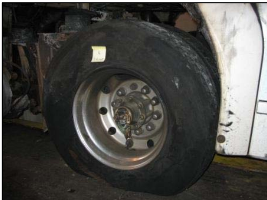
Figure 9. Right outer drive axle tire damage.
