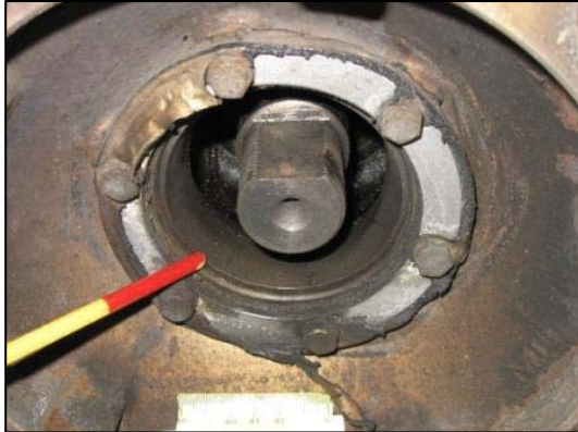
Figure 11. Right tag axle shaft and the wheel bearing races.
