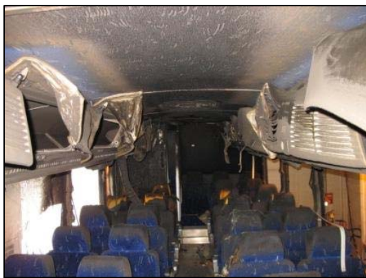
Figure 14. Rearward view of the fire damage to the interior of the motorcoach.
