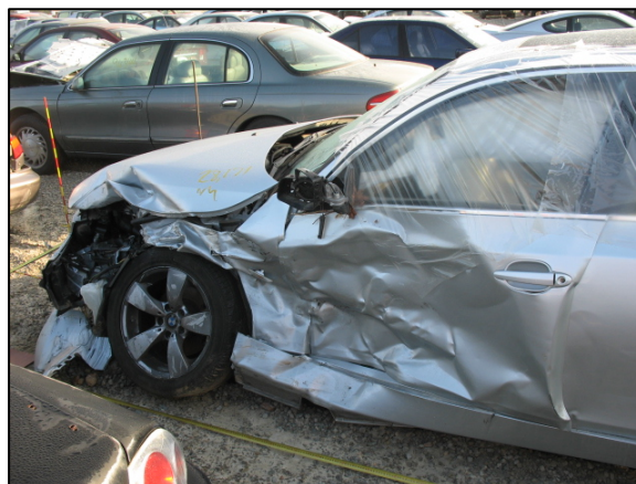
Figure 4: Left side damage sustained by the BMW in the initial impact.
