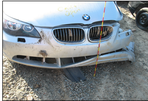
Figure 5: Frontal damage to the BMW resultant to Event 3.
