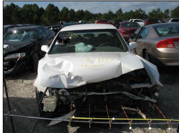
Figure 10: Frontal damage to the Toyota.
