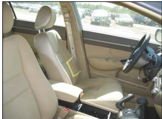
Figure 5: Interior view of the driver seat depicting the seat deformation.
