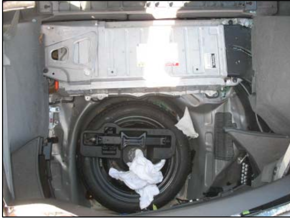
Figure 8: Overhead view into the cargo area depicting the hybrid battery location.
