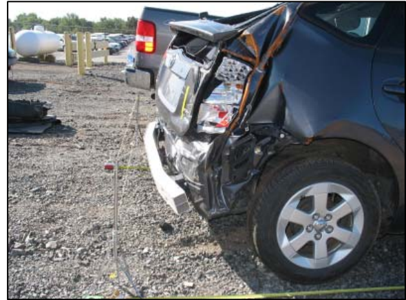
Figure 4: Right lateral view of the depicting the extent of crush at the rear corner.
