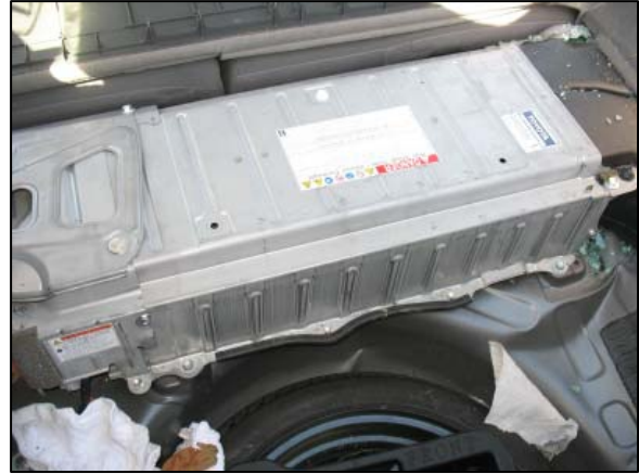
Figure 9: View of the hybrid battery and the buckled floor on right.
