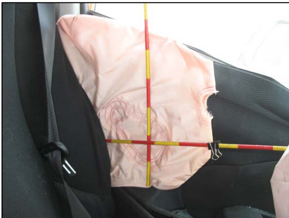
Figure 7: Deployed left side impact air bag.
