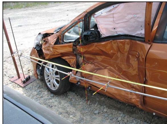
Figure 5: Image depicting the direct contact damage to the left side of the Honda.
