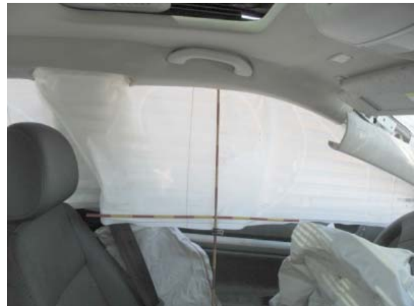
Figure 6: Left IC air bag at the driver's position.
