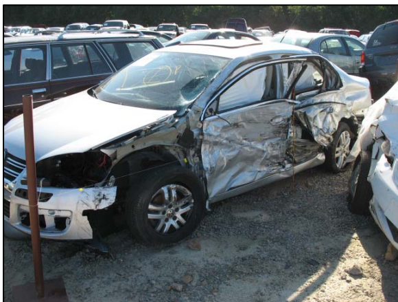
Figure 3: Impact damage to the left side of the Volkswagen.
