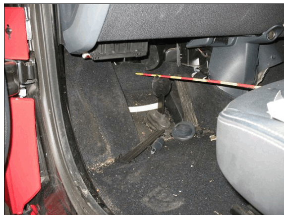
Figure 10: The left toe pan of the Smart intruded 6 cm (2.4 in)
