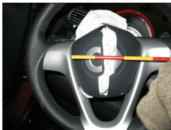
Figure 11: Air bag module cover flaps
