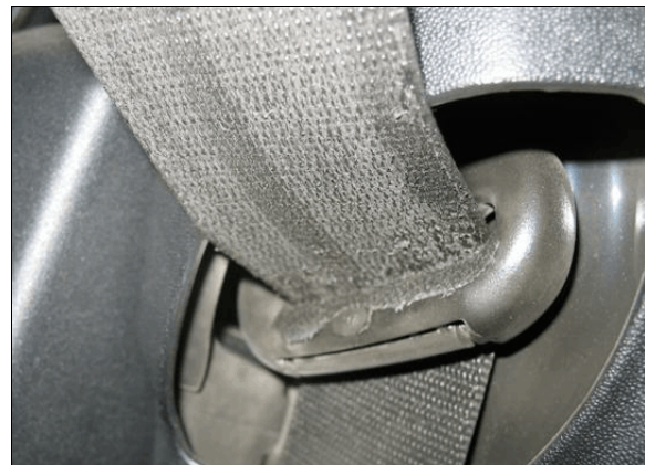
Figure 14: Load abrasion on driver's D-ring and belt webbing
