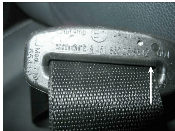
Figure 15: Load abrasions on driver's latch plate belt guide
