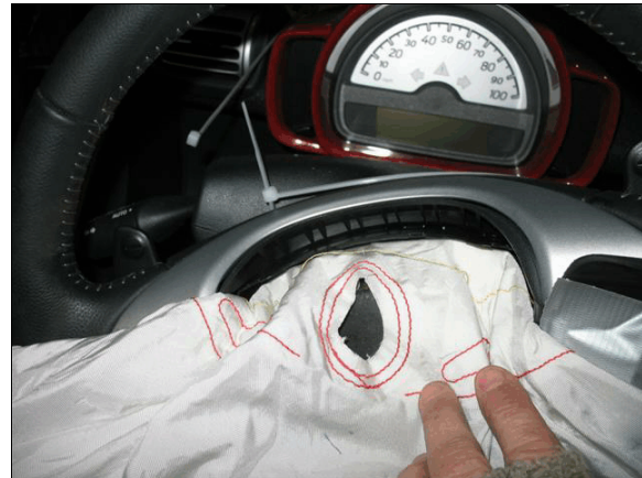
Figure 13: Air bag vent port on the driver's frontal air bag of the Smart
