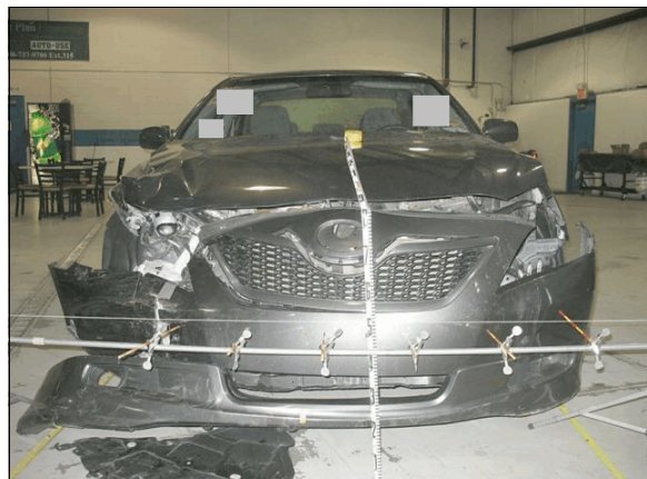
Figure 5: Damage to the front plane of the Toyota from the impact with the front plane of the Smart
