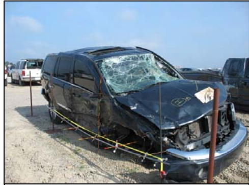
Figure 5: Right side damage to the Aspen.
