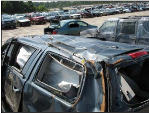
Figure 6: Rollover damage to the left rear of the Aspen.
