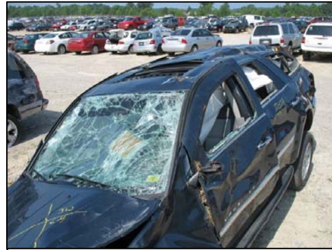
Figure 7: Rollover damage to the left front of the Aspen.
