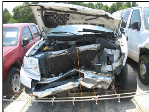
Figure 8: Overall view of the frontal damage to the Ford.
