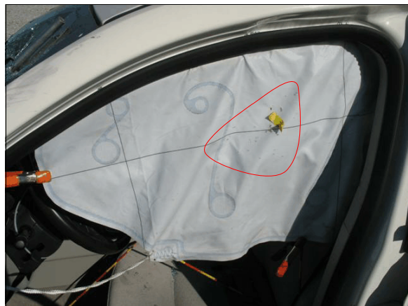
Figure 14: Area of small punctures outlined by red line; punctures caused by flying glass fragments from the disintegrated left front window glazing
