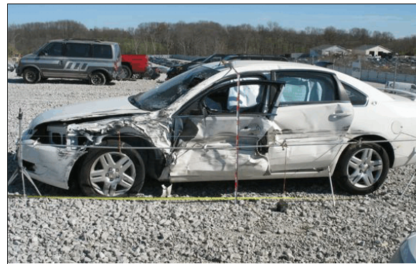
Figure 4: Damage on the left side plane of the Chevrolet from the impact with the Mazda
