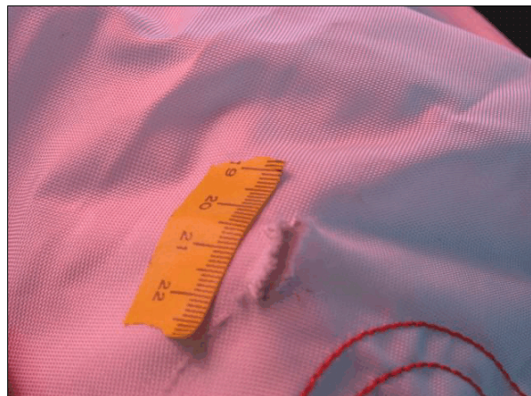
Figure 11: Cut in the fabric of the driver's frontal air bag; cut is near the left vent port
