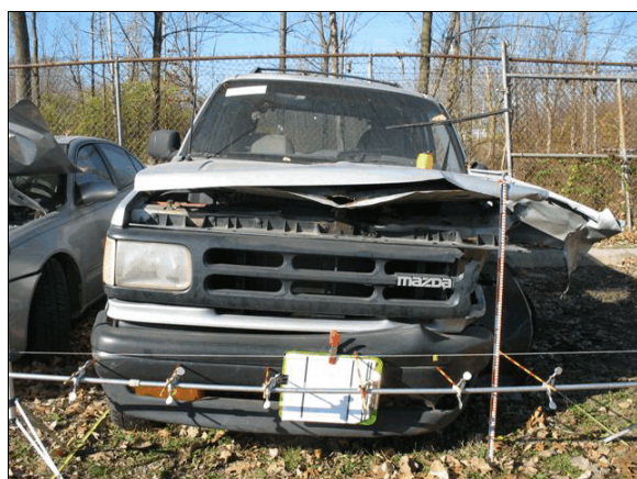
Figure 16: Damage to the front plane of the Mazda
