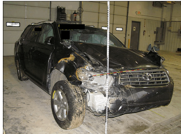
Figure 13: Damage on the front and right side planes from the rollover
