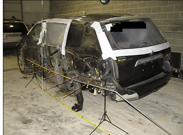
Figure 12: Damage on the left side plane of the Toyota from the impact with the Dodge and the rollover
