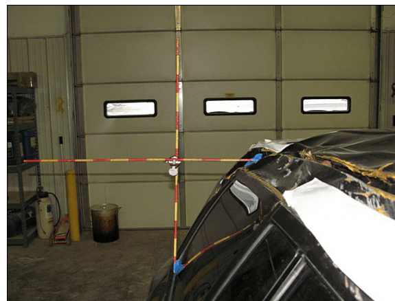
Figure 16: The maximum lateral crush occurred on the right roof side rail immediately forward of the right D-pillar
