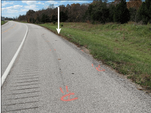
Figure 8: Yaw marks from the right side tires of the Toyota as the vehicle rotated counterclockwise approaching location of rollover initiation (arrow); yaw mark on left is from the left front tire, yaw mark on right is from the right rear tire
