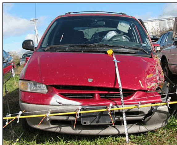
Figure 22: Damage to the front of the Dodge from the impact with the left side plane of the Toyota
