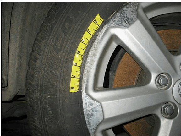
Figure 10: The numbered tape [each increment is 1 in (2.5 cm)] outlines the abrasion on the right front wheel rim due to gouging the bituminous surface of the shoulder
