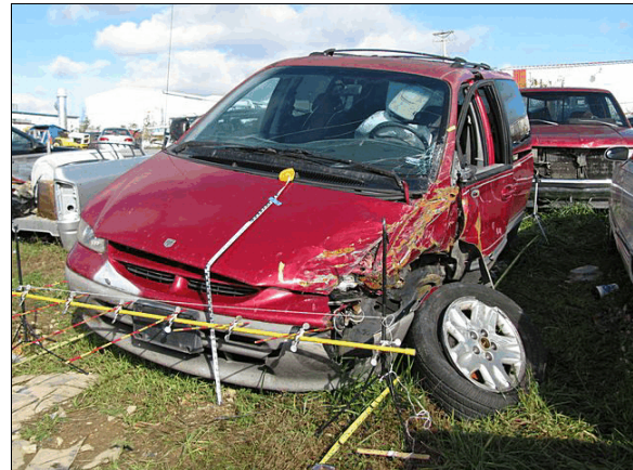
Figure 6: Damage to the front and left side plane of the Dodge from the impact with the left side plane of the Toyota
