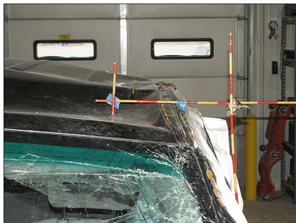
Figure 15: The maximum vertical crush was located on the roof over the driver's seat
