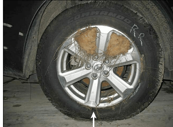
Figure 9: Grass in right rear wheel rim (arrow) from furrowing ground on approach to trip point; dirt in rim is from ground contact during the rollover
