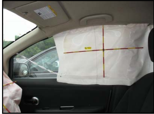
Figure 8: View of the contact evidence to the right curtain.
