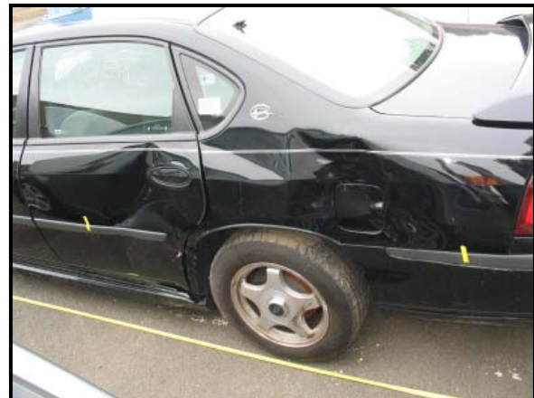
Figure 10: Side slap damage to the left plane of the Chevrolet.
