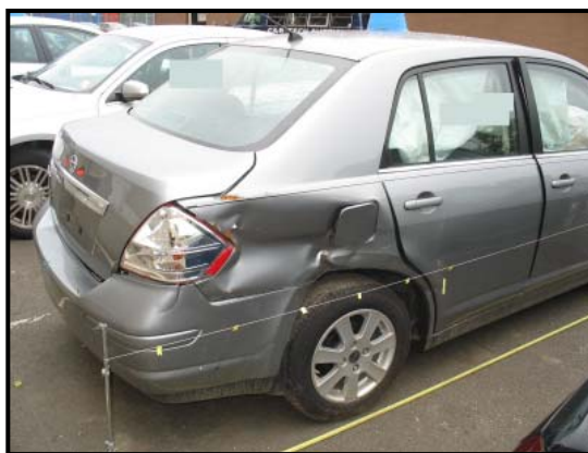
Figure 4: Right rear oblique view of the side slap damage (Event 2).
