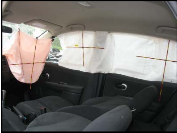
Figure 7: Nissan deployed right curtain.
