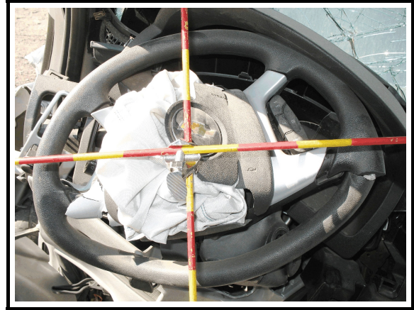
Figure 5. Steering wheel rim deformation
