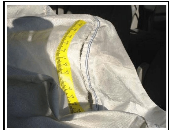
Figure 7. Driver's deployed frontal air bag showing holes at the seam
