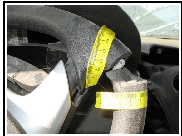
Figure 10. Steering wheel rim showing fracture in left quadrant
