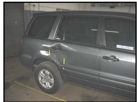
Figure 7: Right side slap damage.
