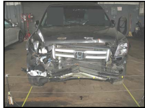
Figure 6: Honda frontal damage.
