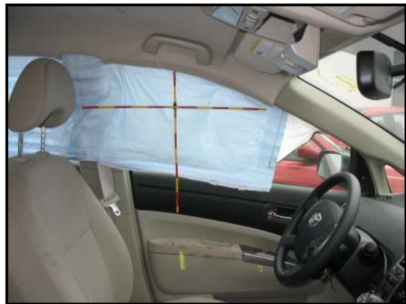
Figure 11: Deployed left inflatable curtain.
