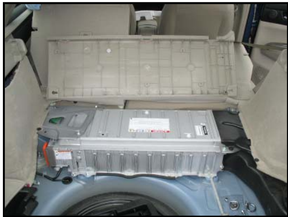
Figure 10: Hybrid battery location.
