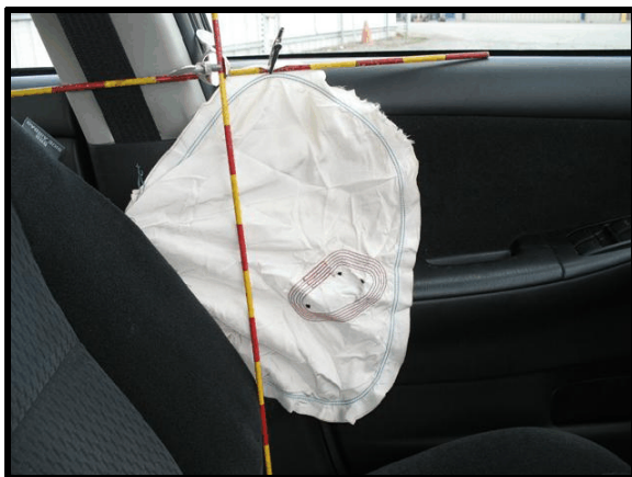
Figure 7. Driver seat-mounted side air bag
