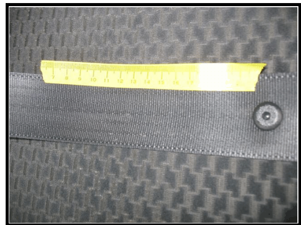
Figure 6. Area of fraying to driver's safety belt webbing
