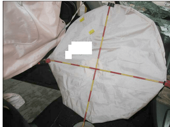
Figure 15: The Honda driver's frontal air bag
