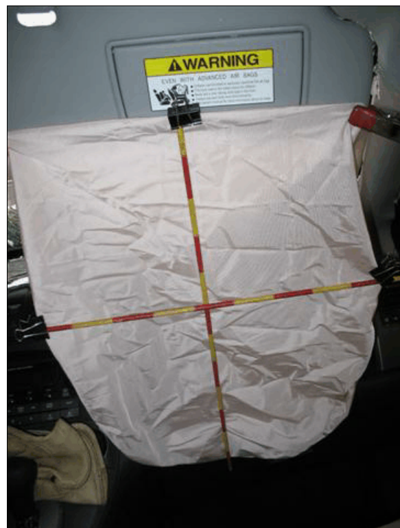
Figure 16: The front passenger's frontal air bag
