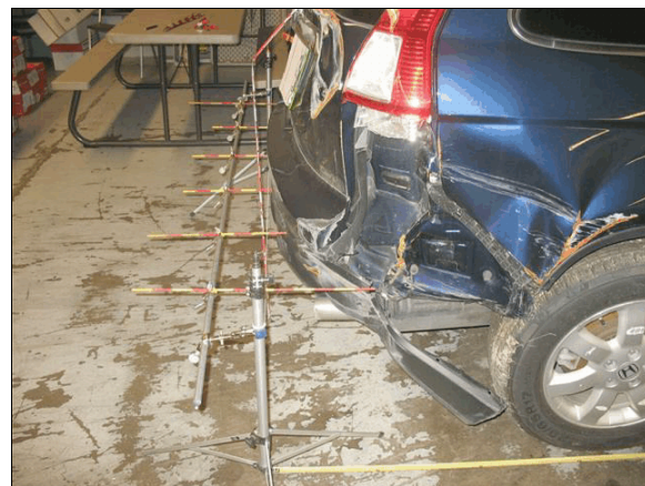
Figure 10: Right side view of the back bumper crush
