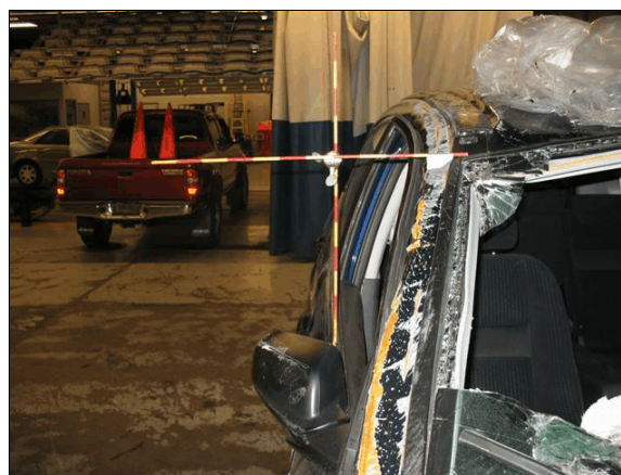
Figure 12: The location of the maximum vertical and lateral crush on the Honda
