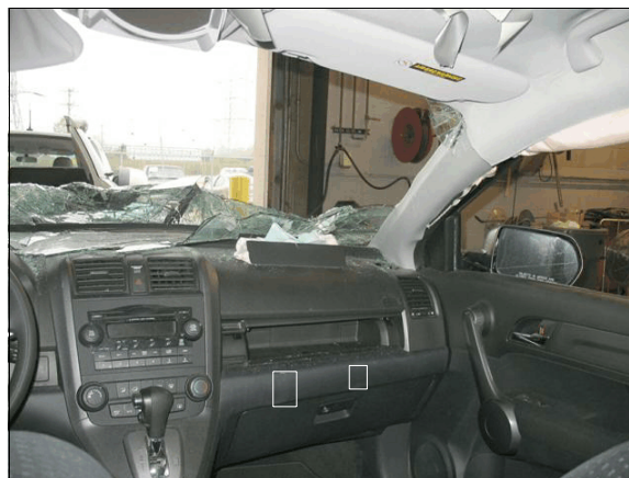
Figure 14: The center and right instrument panel; possible knee contact marks from front passenger highlighted
