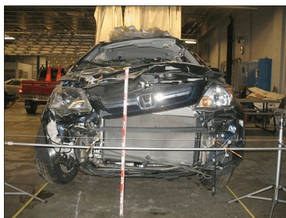
Figure 8: Front plane damage on the Honda from impact with the median barrier
