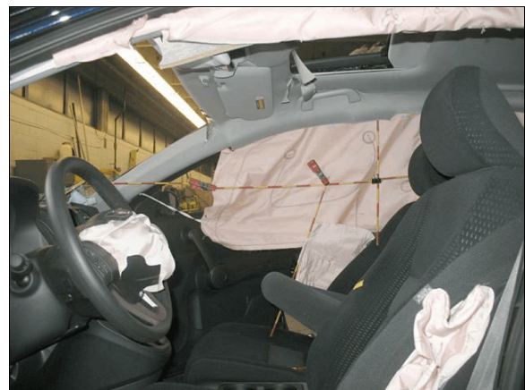
Figure 18: Right IC air bag and passenger seat-mounted side impact air bags
