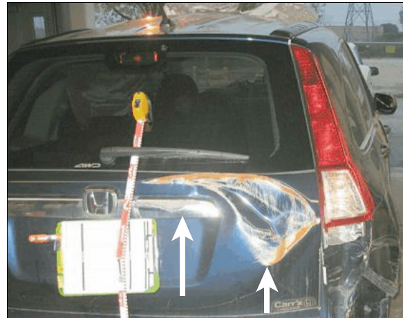
Figure 6: Arrows shows the damage to the tailgate from impact with the median barrier during the rollover (event 5)
