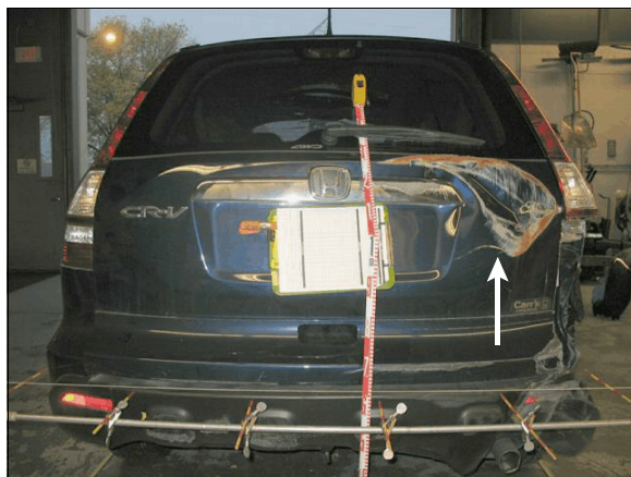
Figure 9: Damage on the Honda’s back bumper from the impact with median barrier; arrow shows the damage on the tailgate that occurred during the rollover
