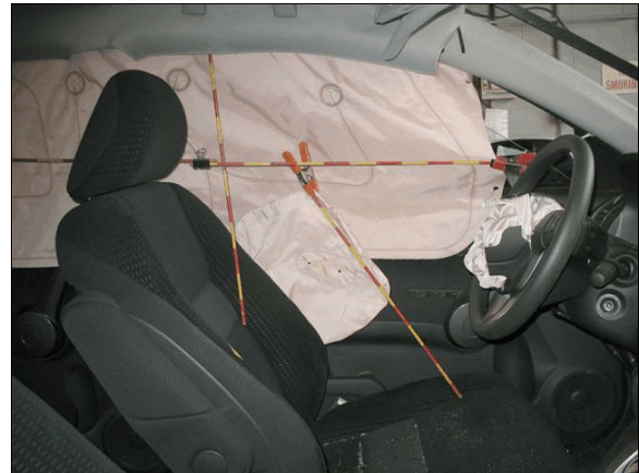
Figure 17: The Honda's left IC air bag and driver's seat-mounted side impact air bags
