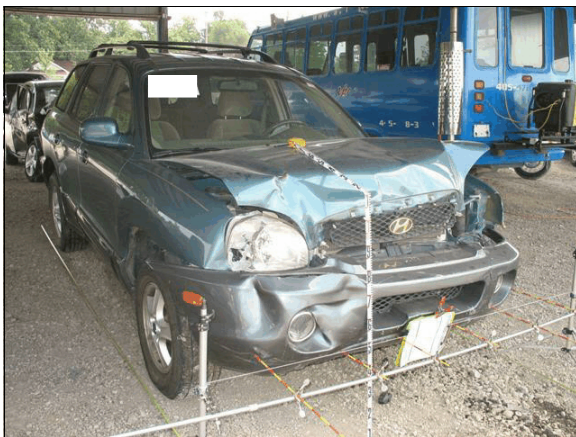
Figure 4: Damage to the front plane of the Hyundai from the impact with the Nissan's left side plane
