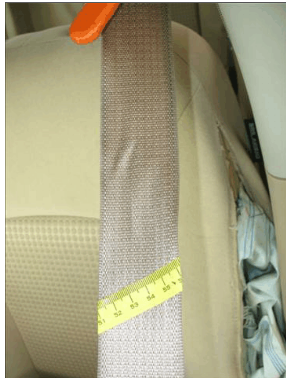
Figure 13: Area on driver's safety belt webbing that was slightly stretched
