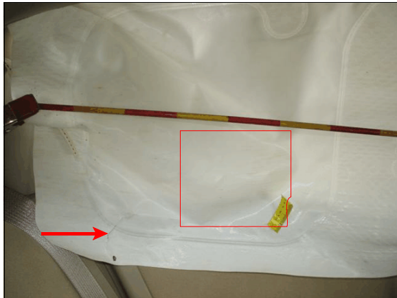
Figure 8: Outline shows area of occupant contact scuff on IC air bag; arrow on left shows location of tear in IC air bag
