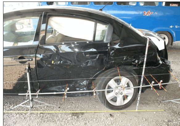
Figure 5: Damage to the left side plane of the Nissan
