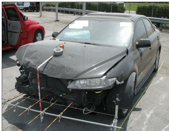
Figure 4: Front plane damage on the Mazda from impact with the right side plane of the Ford
