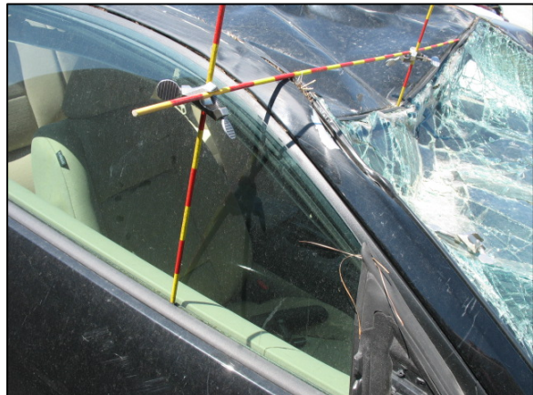
Figure 4: Maximum vertical crush of the roof of the Ford Mustang.
