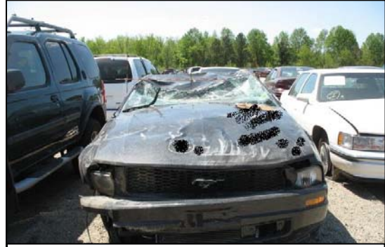
Figure 5: Secondary impact damage to the top of the hood of the Ford Mustang.
