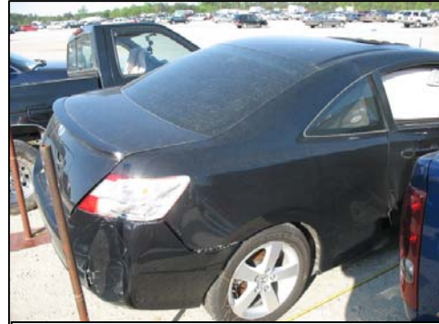
Figure 7: Right rear corner damage.
