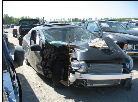
Figure 4: Right front corner damage.
