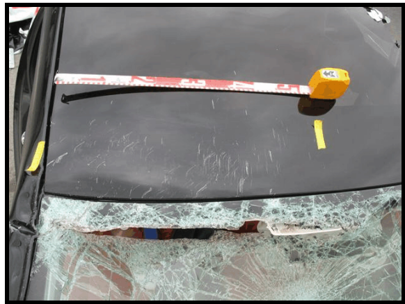
Figure 7. Top rollover damage
