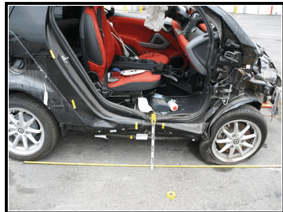
Figure 8. Right side damage
