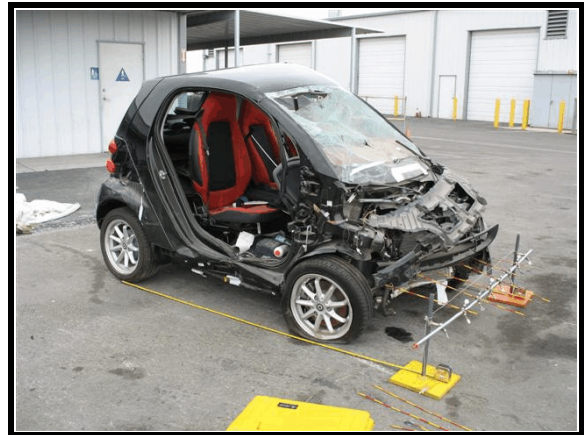
Figure 5. Frontal damage and crush measurement
