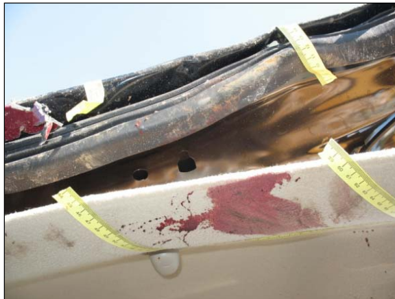
Figure 19: Depicts the headliner and roof side rail contact points associated with the second row left side occupant
