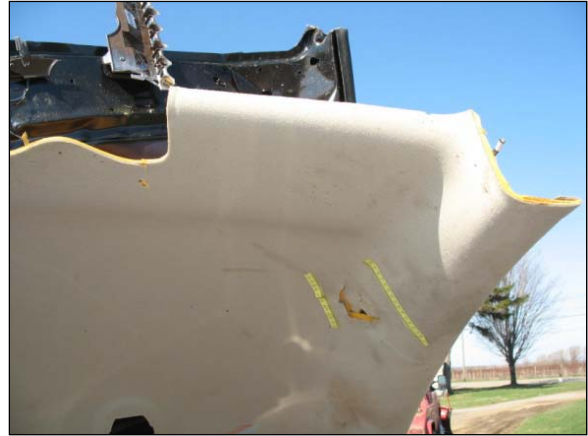
Figure 20: Depicts the headliner contact points associated with the second row right side occupant
