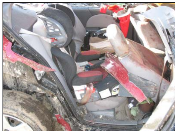
Figure 14: Right lateral interior view of the Saturn depicting the position of the CRS's.
