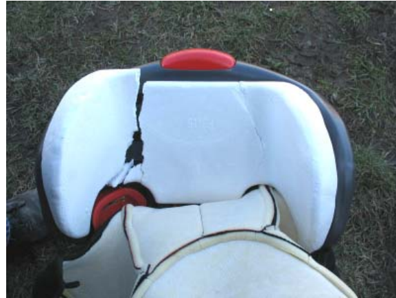
Figure 18: View of the damaged styro-foam insert within the upper back of the Graco CRS.
