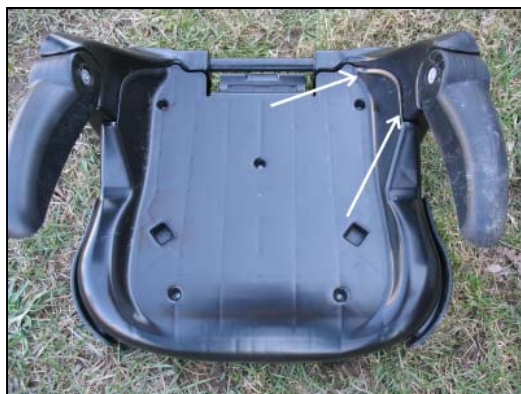
Figure 16: Overhead view of the CRS depicting the loading evidence to the left armrest.
