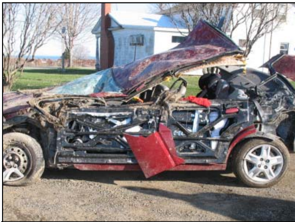
Figure 9: Left side view of the crush to the Saturn's roof area.
