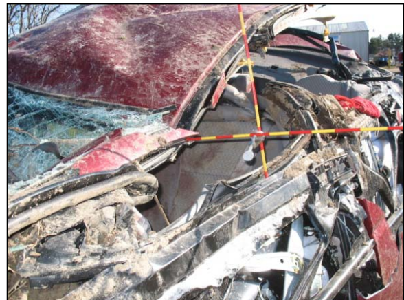
Figure 10: View of the maximum vertical and lateral crush at the Saturn's left A-pillar.
