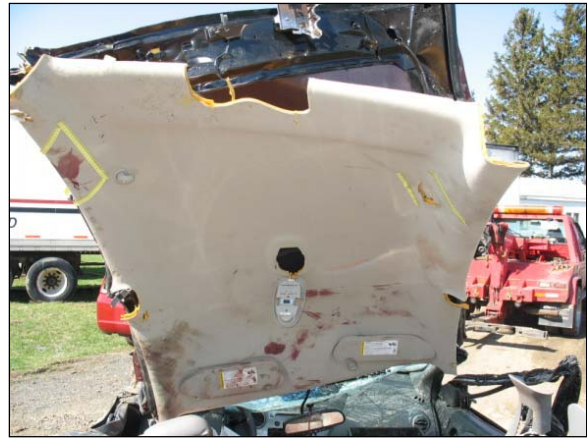
Figure 11: Interior view of the Saturn's headliner and the occupant contacts.
