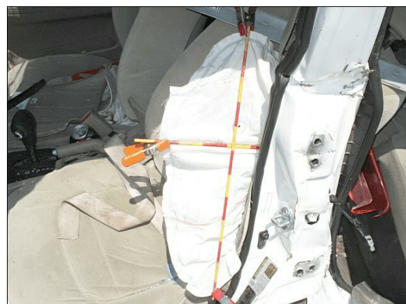
Figure 12: The left front seat back-mounted side impact air bag
