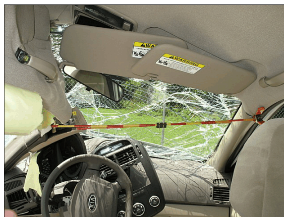
Figure 7: Left A-pillar and roof side rail intrusion into the driver’s occupant space
