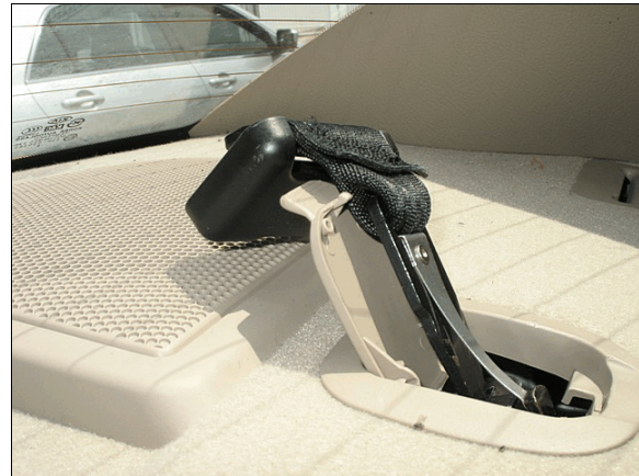
Figure 13: The second row left CSS tether clip was found latched to the upper tether anchor
