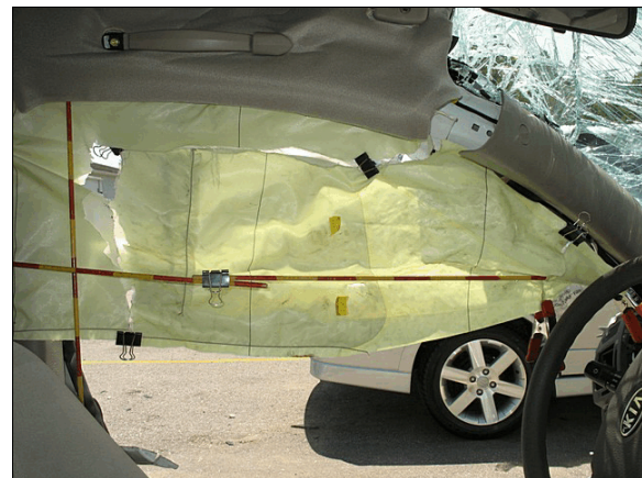
Figure 8: Front portion of the Kia's left IC air bag
