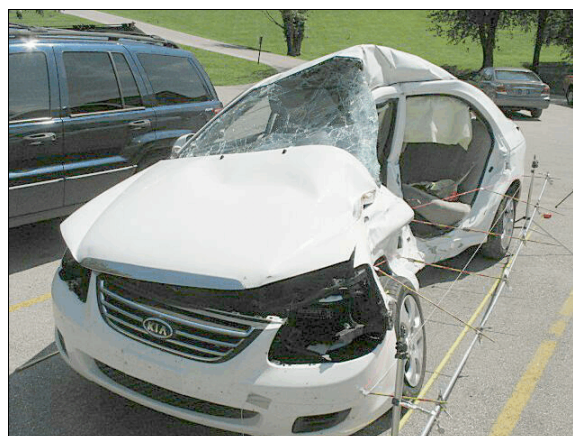
Figure 5: Front left view of Kia's left side crush profile
