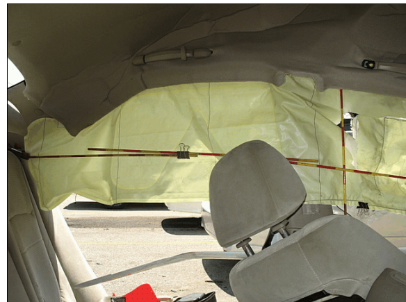
Figure 11: Rear portion of left side curtain air bag
