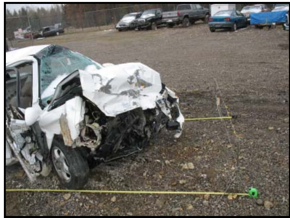
Figure 13: Right lateral view of the frontal deformation.
