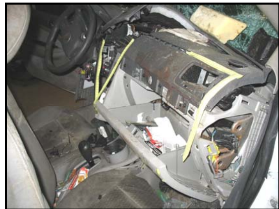
Figure 9: Right instrument panel contact evidence and the non-deployed passenger air bag.
