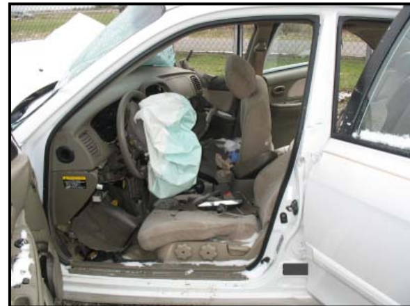
Figure 16: Left lateral view of the Hyundai's intrusion.
