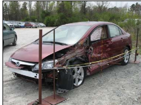
Figure 3: Front left view of the left side damage to the Honda.
