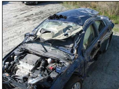
Figure 5: Rollover damage from top left
