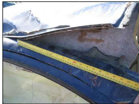
Figure 6: Partial separation of roof body panel
