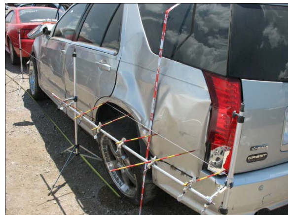
Figure 8: Left side damage from the rollover on the left side plane of the Cadillac
