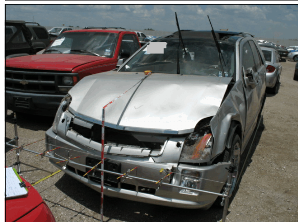
Figure 7: Damage on the front plane, hood, and left side of the Cadillac
