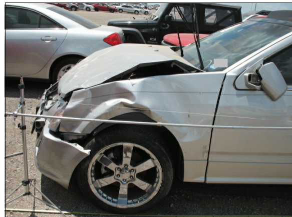
Figure 4: Damage on the grille, hood, and fender of the Cadillac
