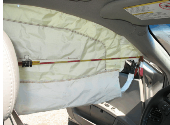
Figure 11: The front left portion of the Cadillac's deployed left IC air bag
