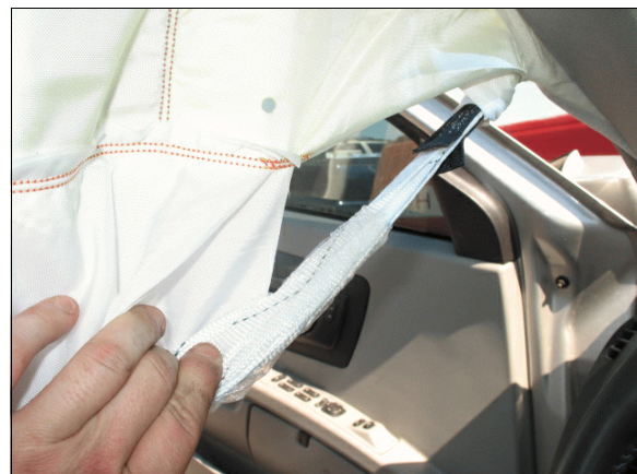
Figure 12: Front tether/air tube of the Cadillac's left IC air bag
