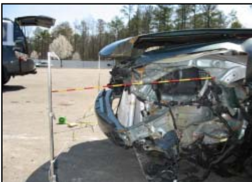
Figure 6. Lateral view of the front ACE frame damage.
