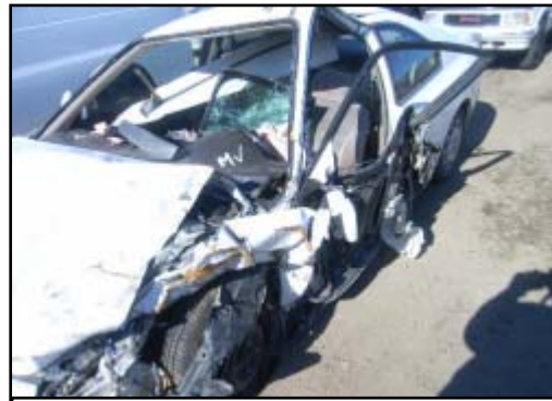
Figure 11. Direct damage extending onto the left door.
