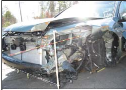
Figure 5. Front left ACE frame damage.
