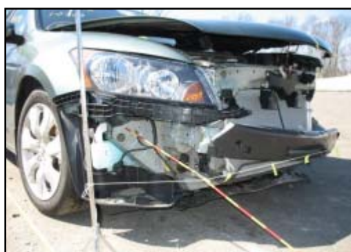
Figure 7. Front right view of the undamaged ACE frame structure.
