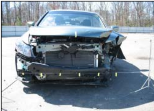
Figure 4. Overall view of the frontal damage.
