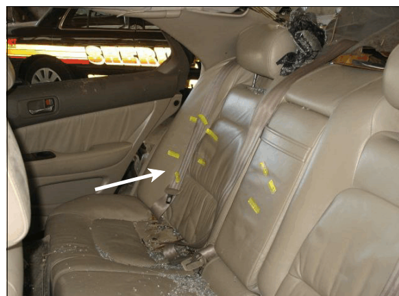
Figure 14: Arrow shows area of scuff marks on the second row right seat that were probably caused by contact with the FSS
