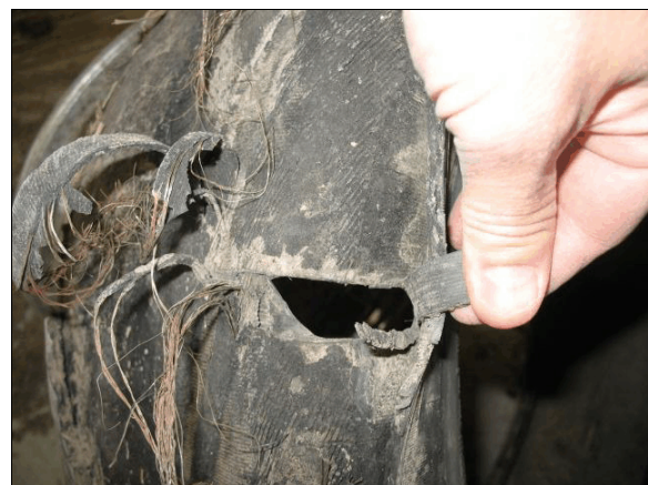
Figure 10: A hole in the tire carcass adjacent to the inside sidewall
