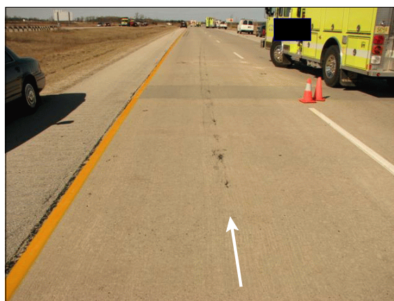
Figure 2: Police on-scene photo showing the travel lane of the Lexus and the beginning of tire marks from the left rear tire
