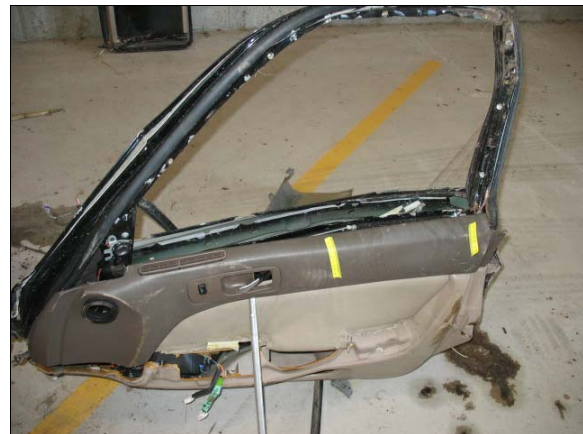
Figure 12: Yellow tape outlines scuff marks on the right front door from contact by the front passenger
