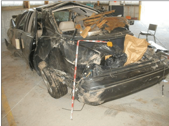
Figure 7: Back left view of the damage on the Lexus
