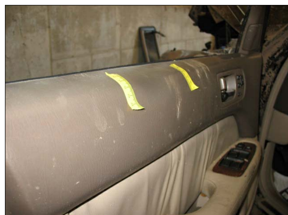
Figure 11: Area of slight deformation on the left front door
