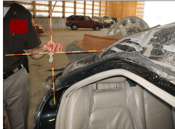
Figure 8: The maximum vertical crush occurred adjacent to the right C-pillar; the maximum lateral crush occurred on the right C-pillar
