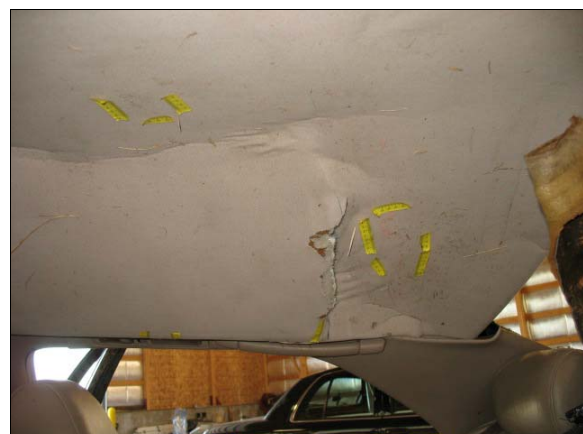
Figure 13: Scuff marks and damage on the roof at the second row right seat position
