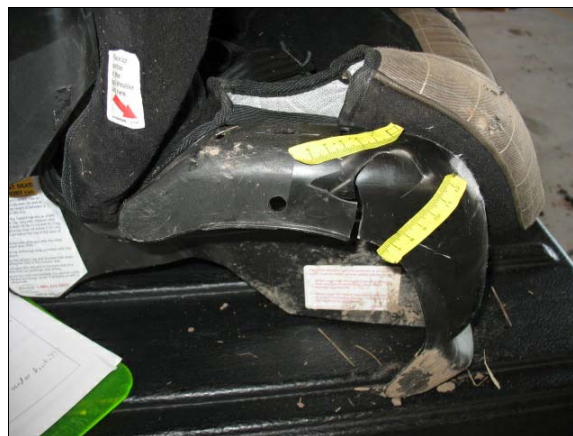
Figure 17: Cracks in the plastic on the right arm rest
