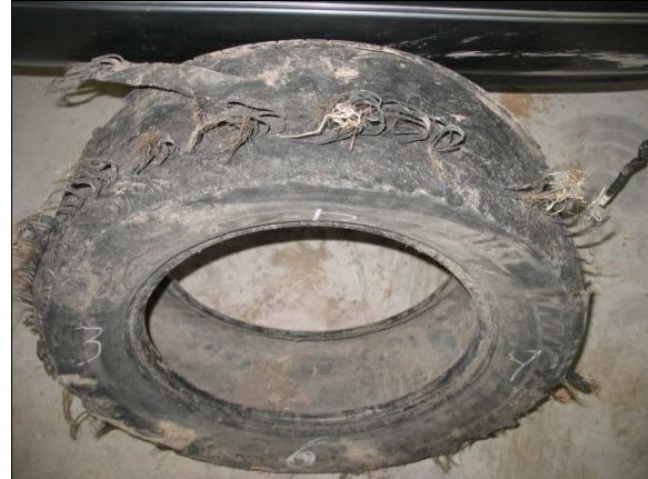
Figure 3: The tread separated from the left rear tire
