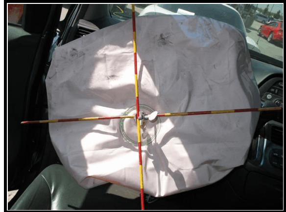
Figure 11. Driver's air bag
