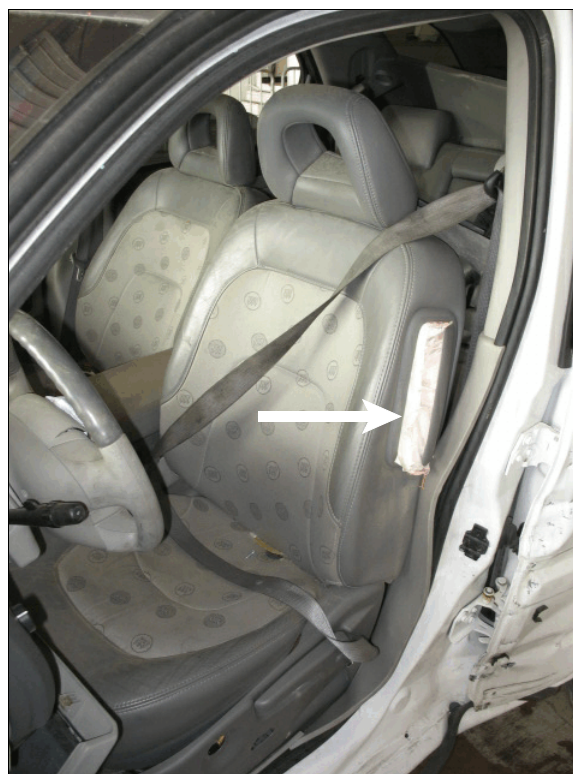
Figure 8: The driver's seat; arrow shows the packed seat-mounted side impact air bag and the module cover flap
