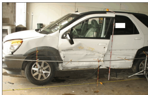
Figure 4: Damage to the left side plane of the Rendezvous from the impact with the Century
