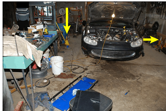
Figure 5: Arrows show three of the four jack stands that were in the immediate vicinity of the vehicle
