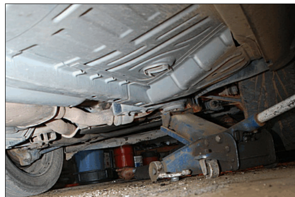
Figure 6: The floor jack was positioned under the right frame member, behind the right front wheel
