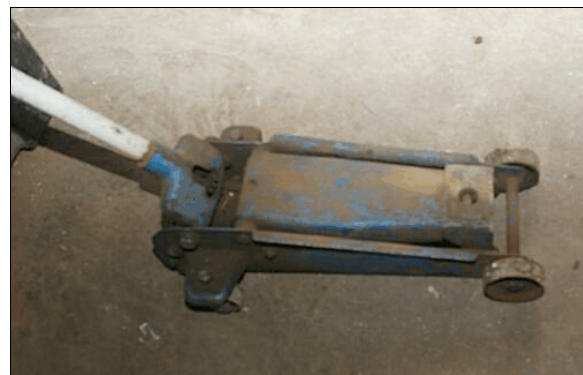
Figure 3: The floor jack used by the victim to raise the front of the Chrysler; the make and model could not be determined
