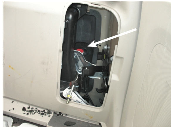
Figure 12: Inertia activated high voltage shut off switch in rear right side of Escape
