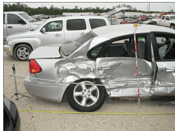
Figure 5: Damage to the Taurus' right side plane from the impact with the Escape
