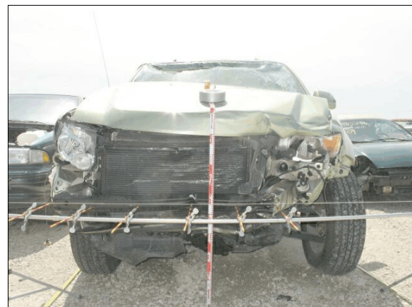
Figure 4: Damage to the Escape's front plane from the impact with the Taurus
