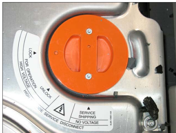
Figure 9: The high voltage service disconnect switch; switch in the locked position at inspection
