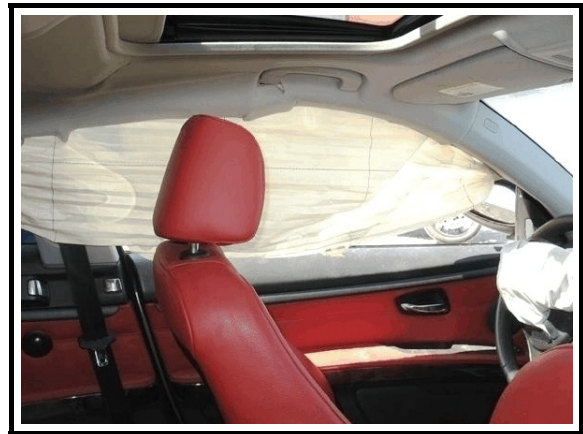
Figure 7. Deployed left IC air bag
