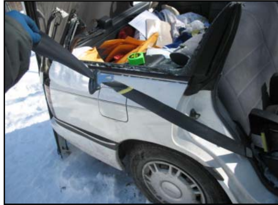
Figure 10: Rear right safety belt webbing.
