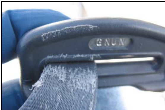
Figure 11. Frictional abrasions of the rear right latch plate.
