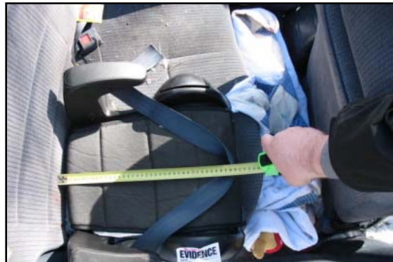
Figure 12. Loose fit of the lap belt webbing.
